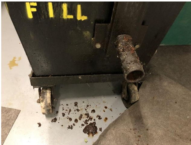
Figure 8: Grease spilled and covered with dry rite instead of cleaning it up.
