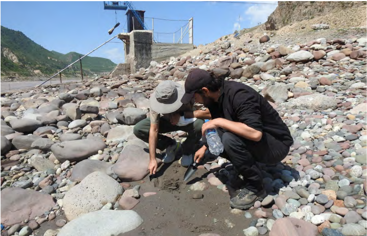
MSRI Scientists collecting sediment samples from the Vakhsh River as part of the World Bank funded project to study sediment loads to Nurek Dam, the largest hydropower station in Tajikistan.
